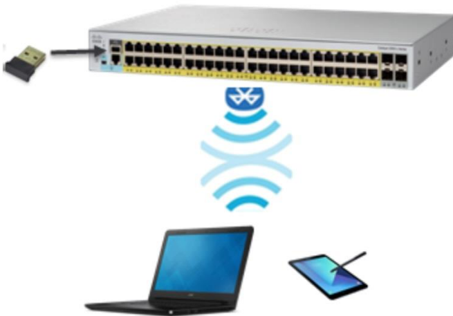
Figure 4. Over-the-air switch access using Bluetooth
